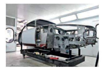
Objective – to remove all components, filth, materials, coverings and paint which are required prior to separation of the outer body shell from the chassis assembly. First stage of the strip is to remove all interior trim and glass, labelling and carefully storing. Next follows bumpers, all bright trim, light fittings etc. Next the transmission tunnel is removed followed by the removal of radiators, engine and transmission in unit, initially to be stored and later assessed.
